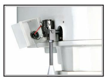
Figure 69. Spindle brake switch wiring.
